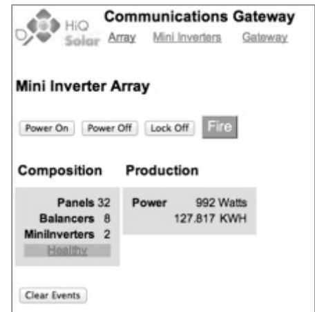
Figure 33: Web interface for the Gateway showing array statistics
