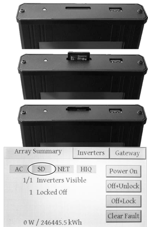
Figure 41: Symptoms of a missing or not fully engaged memory card
