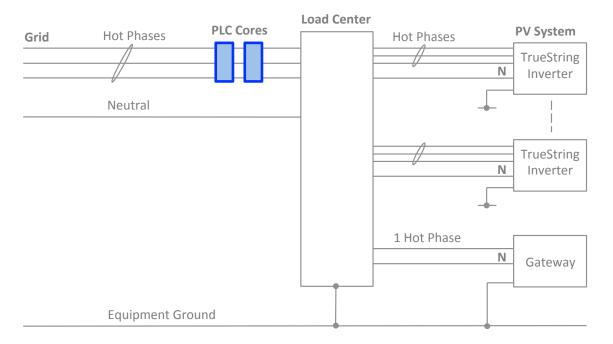
Note that for the Cores to achieve the desired affect, all three hot phases must pass through the same core(s), and the Neutral and Ground MUST NOT. We recommend a minimum of two cores be used, although more may be added if desired and there is sufficient physical space.
