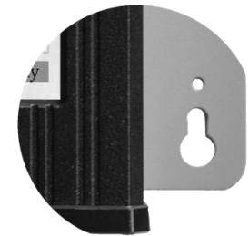
Figure 6: Gateway baseplate showing keyhole mounting and drilling guide hole.
