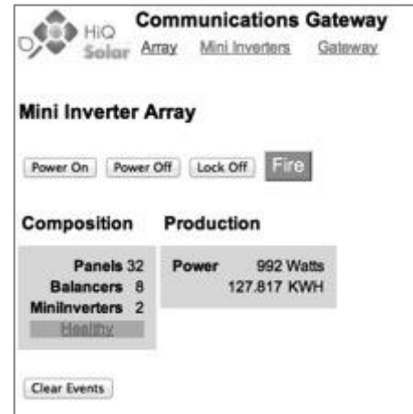
Figure 31: Web interface for the Gateway showing array statistics
