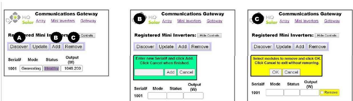
Figure 25 Adding and Removing Inverters using Web Interface
