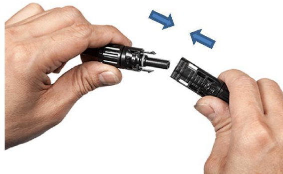
Figure 11 Connecting PV Plugs
